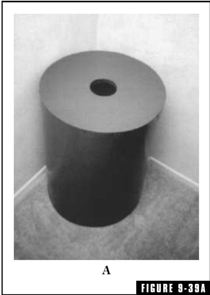
Typical Helmholtz resonator made of readily available materials.
